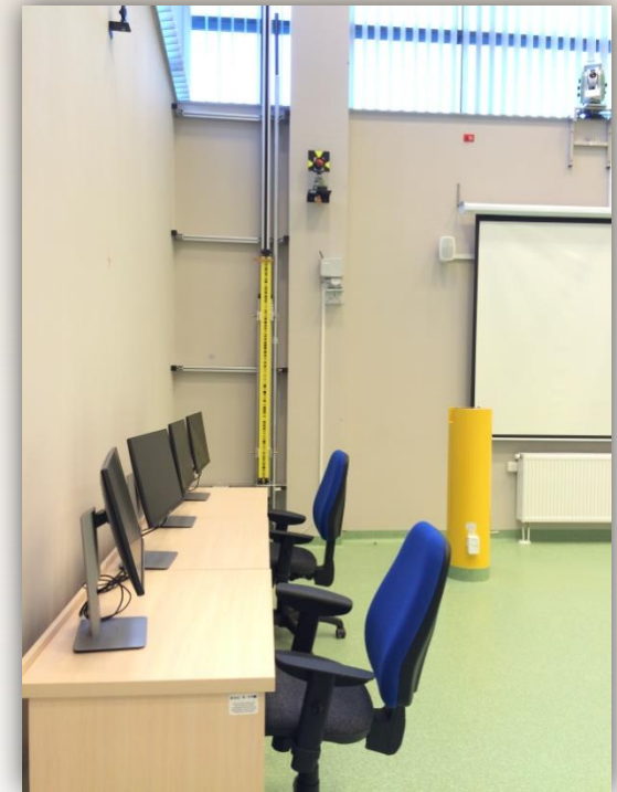
Vertical comparator of leveling staff – designed to control height differences heights measurements and accuracy of leveling staffs. Using laser interferometer LS10.
