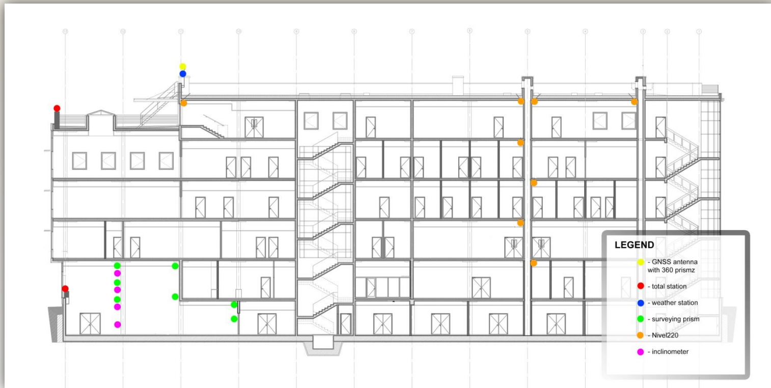
Leica GeoMoS – sensor location – GEO-INFO-HYDRO building
