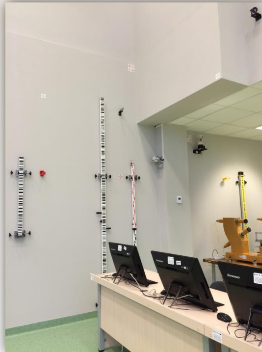
Precise level staffs installed in the laboratory
