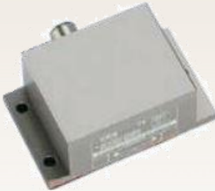
Tiltmeter KELAG SCA124T Measuring tilt in real time Range - +/- 30 degrees Resolution – 0,03 degree Installed in inclinometer tube
