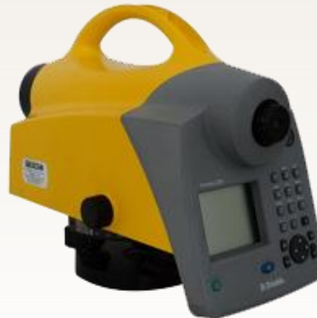
Trimble DiNi 0,3 Precise code level Model instrument to measure height differences
